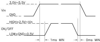
Until Vin voltage reaches the spec voltage, it does not change  ${\sf ON/OFF}$  function from LOW to HIGH.
