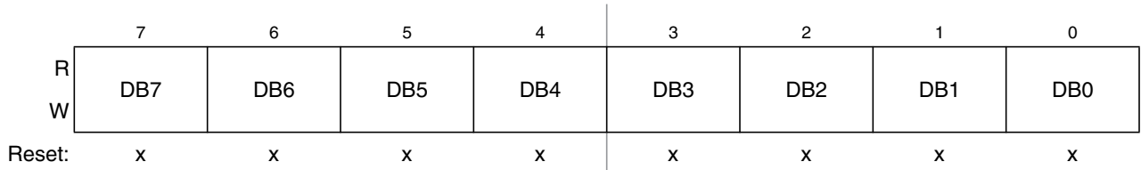
Figure 10-33. Data Segment Registers (DSR0–DSR7) — Extended Identifier Mapping
