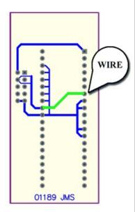
Modification for the 28-pin SOIC ZIF Adapter (Part # 28SOIC)
