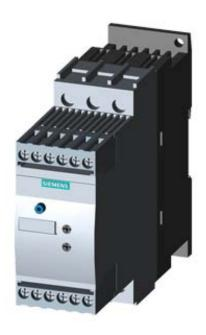
SIRIUS SOFT STARTER, SIZE S0, 38A, 18.5KW/400V, 40 DEGREES, 200-480V AC, 110-230V AC/DC, SCREW TERMINALS
