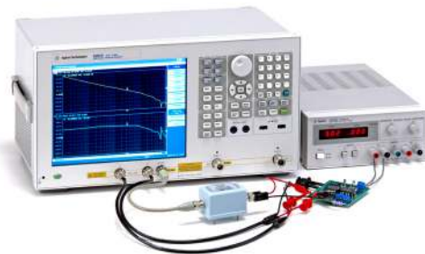
Pomona 3787-C-18 test lead (connected to gain-phase receiver ports) Pomona 2886 BNC breakout (connected to 0017CC)
