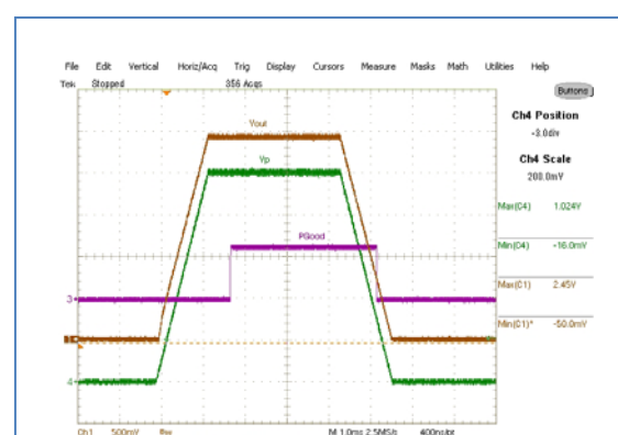
Figure 44: Voltage tracking using Vp pin Ch1:V out , Ch2: P Good , Ch3:V p
