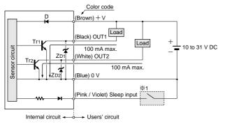
Symbols ... D: Reverse supply polarity protection diode Z<sub>D1</sub>, Z<sub>D2</sub>: Surge absorption zener diode Tr1, Tr2: NPN output transistor
