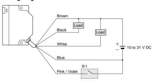
Non-voltage contact or NPN open-collector transistor
