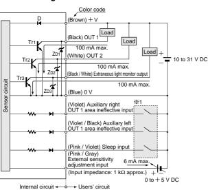
Symbols ... D: Reverse supply polarity protection diode Z<sub>D1</sub>, Z<sub>D2</sub>, Z<sub>D3</sub>: Surge absorption zener diode Tr<sub>1</sub>, Tr<sub>2</sub>, Tr<sub>3</sub> : NPN output transistor
