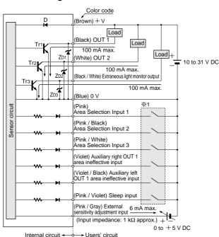
Symbols ... D: Reverse supply polarity protection diode Z<sub>D1</sub>, Z<sub>D2</sub>, Z<sub>D3</sub>: Surge absorption zener diode Tr<sub>1</sub>, Tr<sub>2</sub>, Tr<sub>3</sub>: NPN output transistor
