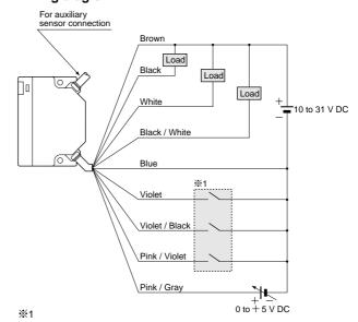
Non-voltage contact or NPN open-collector transistor
