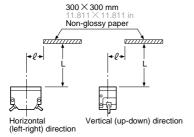
Note: The sensitivity has been adjusted so that the maximum sensing range for white non-glossy paper (300  $\times$  300 mm 11.811  $\times$  11.811 in) is 3 m 9.843 ft (1 m 3.281 ft for PX-21 and PX-23ES, 5 m 16.404 ft for PX-26) with the L, C and R areas effective.
