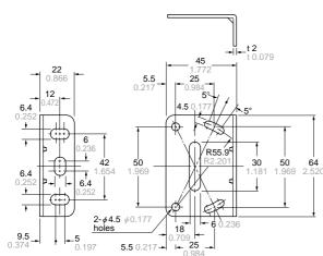
Material: Cold rolled carbon steel (SPCC)(Uni-chrome plated)
