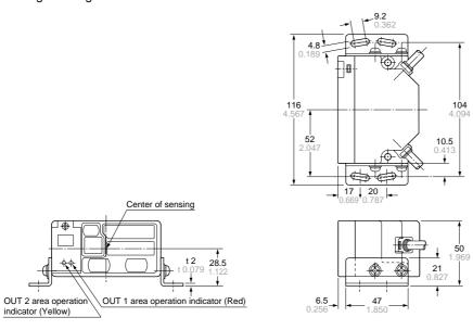
DIMENSIONS (Unit: mm in) The CAD data in the dimensions can be downloaded from the SUNX website: http://www.sunx.co.jp/
