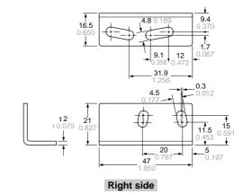
Material: Cold rolled carbon steel (SPCC)
