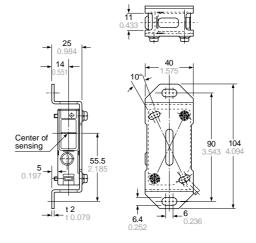
Material: Cold rolled carbon steel (SPCC)(Uni-chrome plated)
