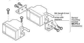
• The tightening torque for PX-SB1 (auxiliary sensor) should be 0.8 N·m or less.
