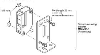
• Mount the sensor, horizontally, at least 300 mm 11.811 in above the floor, to avoid reflection from the floor.
