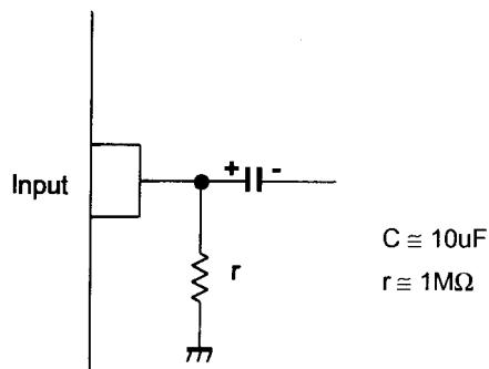
This IC requires  $0.1\mu F$  capacitor between INPUT and GND,  $1M\Omega$  resistance between INPUT and GND for clamp type input at mute mode.
