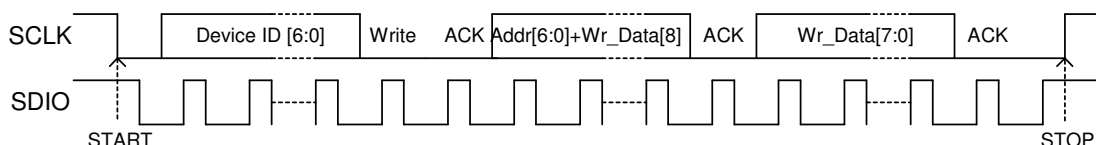
Figure 23: Write Sequence(writing 1 register)
