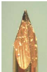
Standard Gold Coating, Contamination after 1/2 Mio contacts
