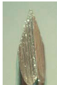
FEINMETALL „Progressive Coating“, Contamination after 1/2 Mio contacts
