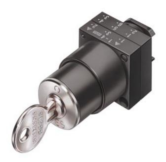
22MM PLASTIC ROUND ACTUATOR: CES KEY-OPER.SWITCH WITH 2 KEYS 3 SWITCH POSITIONS I-O-II LATCHING LOCK NO SSG 10, REMOVAL POS. O WITH HOLDER
