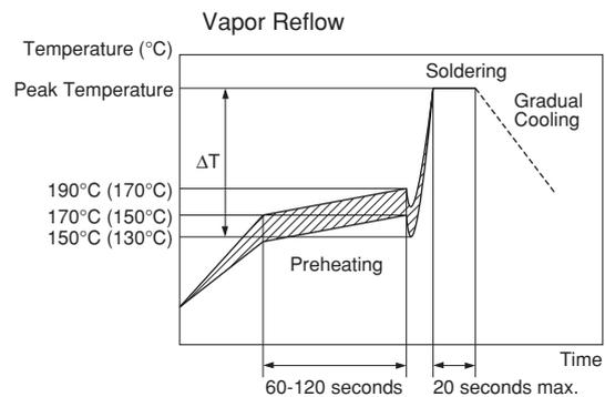
**[Allowable Reflow Soldering Temperature and Time]**
