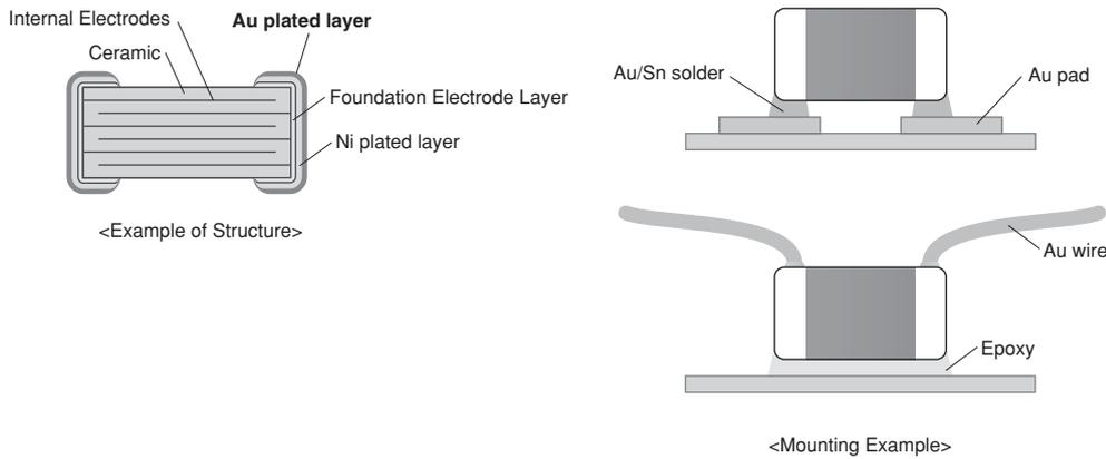
**2 Ideal for mounting in packages, such as optical communication related devices , IC and etc.**
