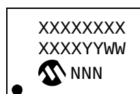
8-Lead SOIC (150 mil)
