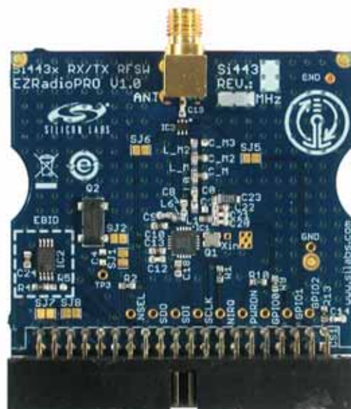
Figure 17. Single-Ended TX and RX Testcard
