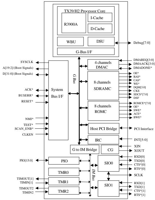
\*Note: This diagram shows the full set of functional signal connections. Due to pin multiplexing, not all of these signals will be available.
