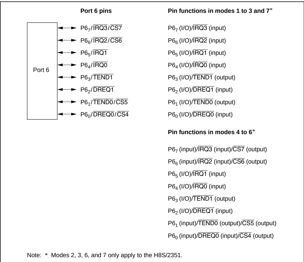
Figure 9.6 Port 6 Pin Functions
