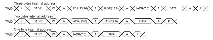
Figure 24-12. Master Read with One, Two or Three Bytes Internal Address and One Data Byte
