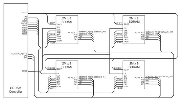
Figure 28-3. SDRAM Controller Connections to SDRAM Devices: 16-bit Data Bus Width
