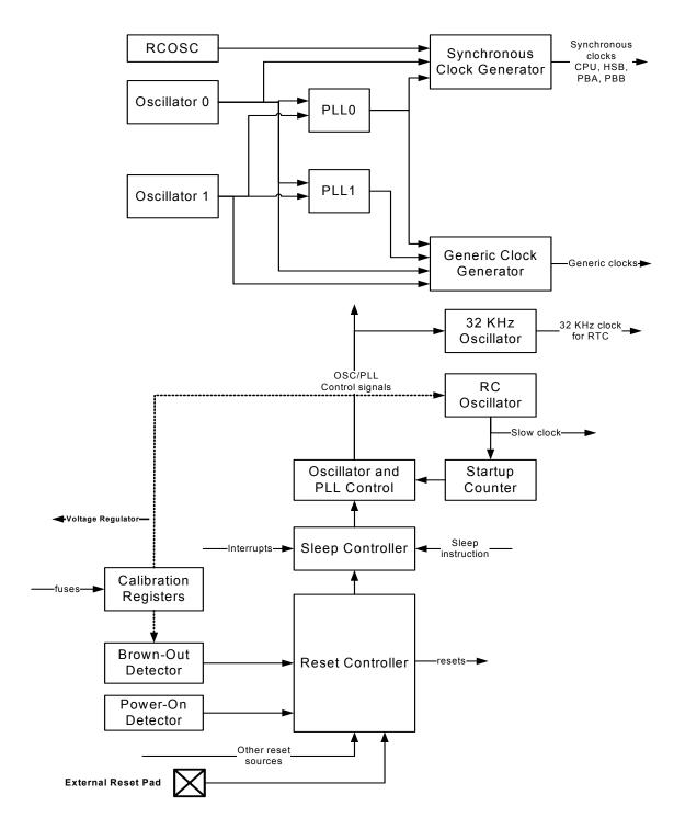
Figure 13-1. Power Manager block diagram
