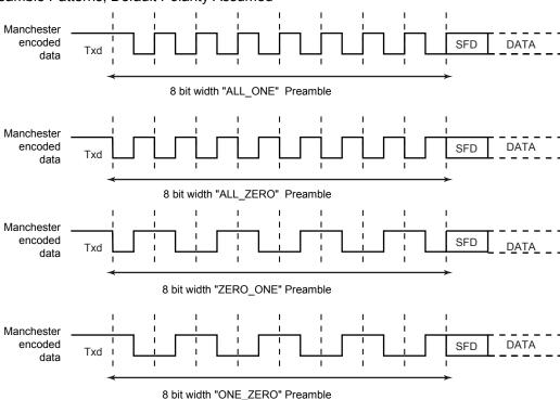
Figure 26-9. Preamble Patterns, Default Polarity Assumed
