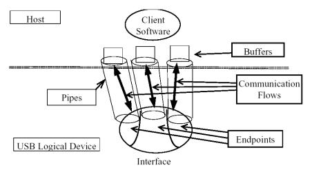
In host mode, the USB controller associates a pipe to a device endpoint, considering the device configuration descriptors.
