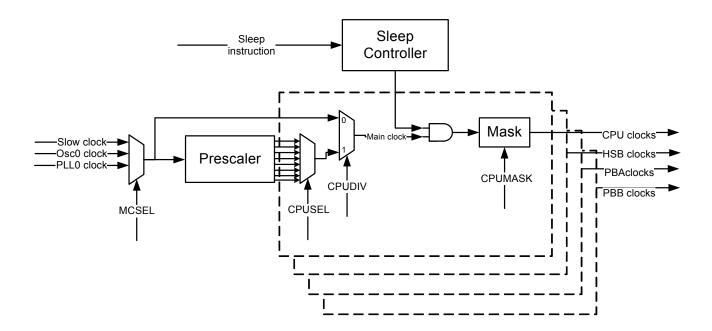
Figure 13-4. Synchronous clock generation
