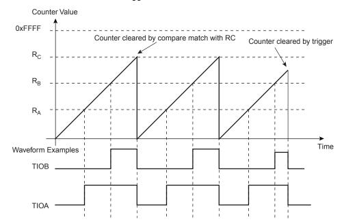
Figure 31-9. WAVSEL = 10 With Trigger
