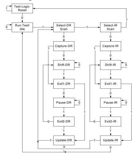
Figure 36-2. TAP Controller State Diagram
