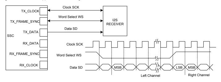
Figure 25-18. Codec Application Block Diagram
