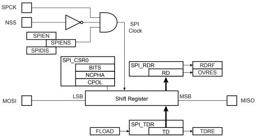
Figure 23-9. Slave Mode Functional Block Diagram
