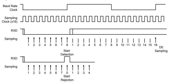
Figure 26-13. Asynchronous Character Reception
