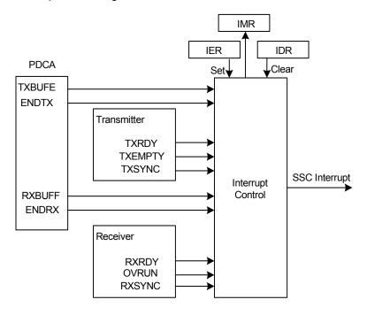
Figure 25-16. Interrupt Block Diagram
