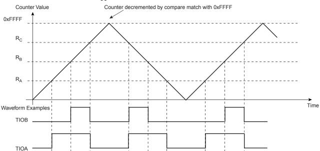
Figure 31-10. WAVSEL = 01 Without Trigger
