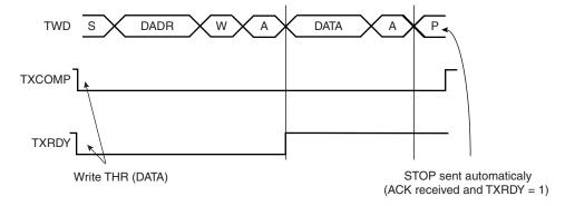
Figure 24-7. Master Write with Multiple Data Byte
