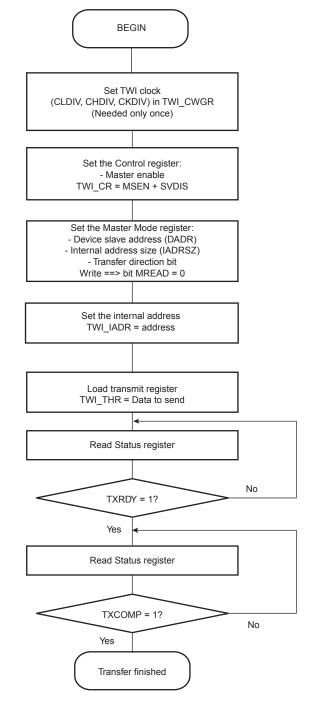
Figure 24-14. TWI Write Operation with Single Data Byte and Internal Address
