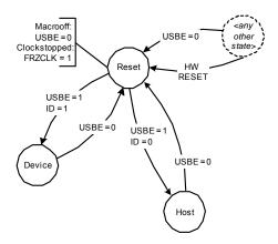
After a hardware reset, the USB controller is in the Reset state. In this state:
