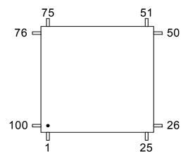
Table 7-1. TQFP100 Package Pinout
