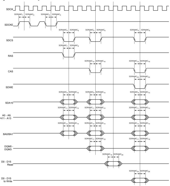
Figure 38-4. SDRAMC Signals relative to SDCK.
