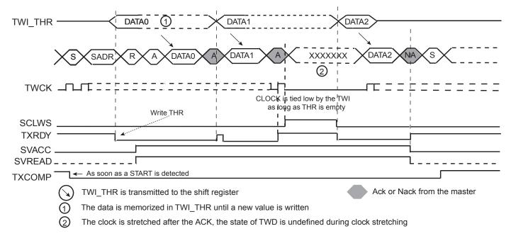
Notes: 1. TXRDY is reset when data has been written in the TH to the shift register and set when this data has been acknowledged or non acknowledged.
