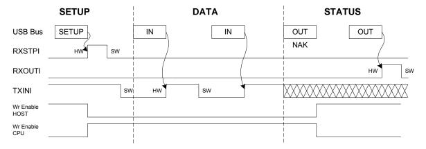
A NAK handshake is always generated on the first status stage command.
