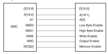
Figure 27-6. Memory Connection for a 32-bit Data Bus
