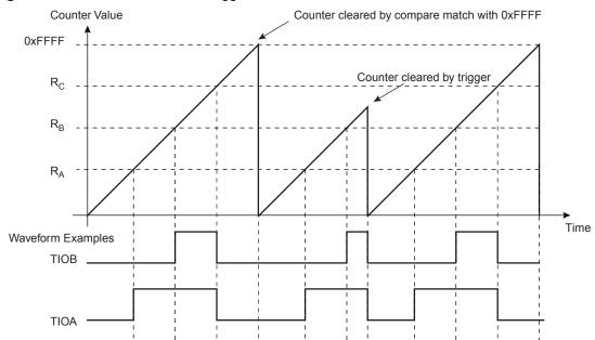
Figure 31-7. WAVSEL= 00 with trigger
