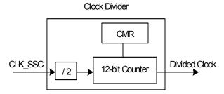
The Master Clock divider is determined by the 12-bit field DIV counter and comparator (so its maximal value is 4095) in the Clock Mode Register CMR, allowing a Master Clock division by up to 8190. The Divided Clock is provided to both the Receiver and Transmitter. When this field is programmed to 0, the Clock Divider is not used and remains inactive.
