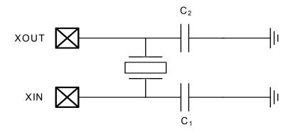
Figure 13-2. Oscillator connections
