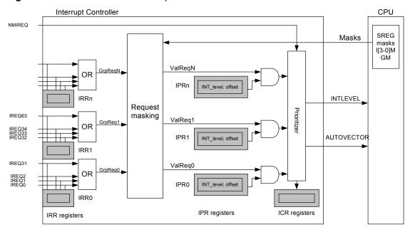
Figure 16-1. Overview of the Interrupt Controller
