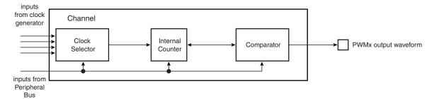
Each of the 7 channels is composed of three blocks:
