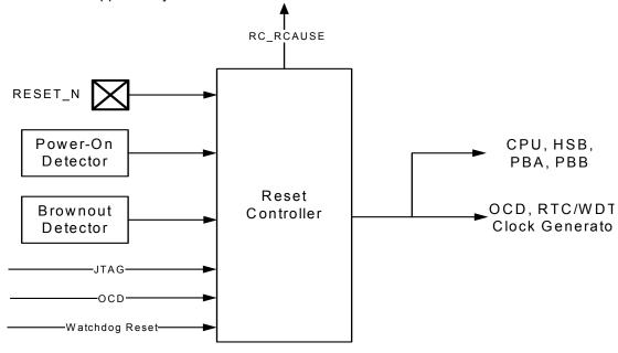
Figure 13-6. Reset Controller block diagram
