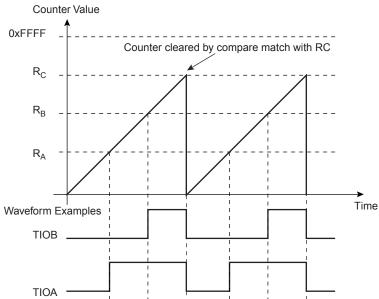
**Figure 31-8.** WAVSEL = 10 Without Trigger
