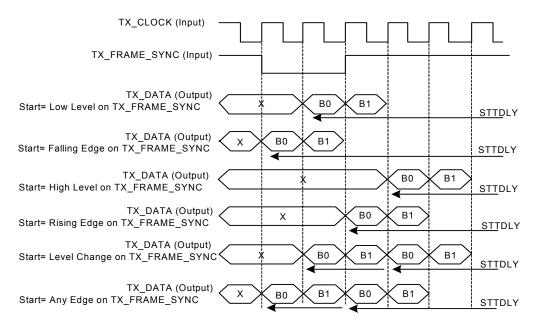
Figure 25-11. Receive Pulse/Edge Start Modes
