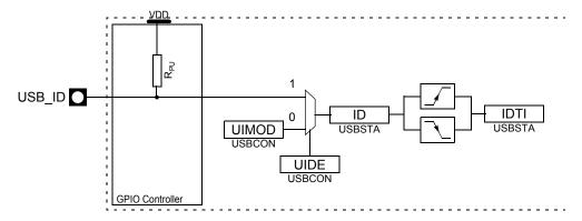
The USB mode (device or host) can be either detected from the USB\_ID pin or software selected from the UIMOD bit, according to the UIDE bit. This allows the USB\_ID pin to be used as a general purpose I/O pin even when the USB interface is enabled.
