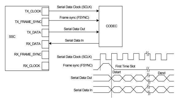
Figure 25-19. Time Slot Application Block Diagram
