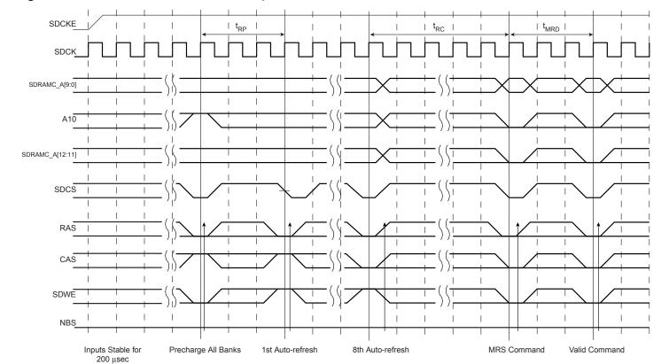
Figure 28-4. SDRAM Device Initialization Sequence
