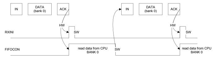
Figure 30-26. Example of an IN Pipe with 2 Data Banks
