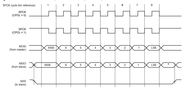
Figure 23-3. SPI Transfer Format (NCPHA = 1, 8 bits per transfer)
