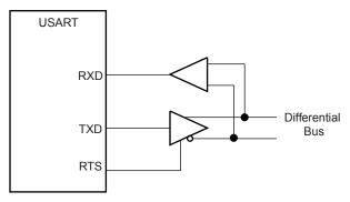
The USART is set in RS485 mode by programming the MODE field in the Mode Register (MR) to the value 0x1.
