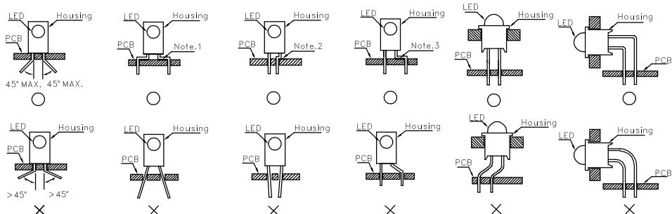
"○" Correct mounting method "X" Incorrect mounting method
