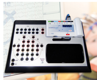
Stationary system for long-term EEG recordings
