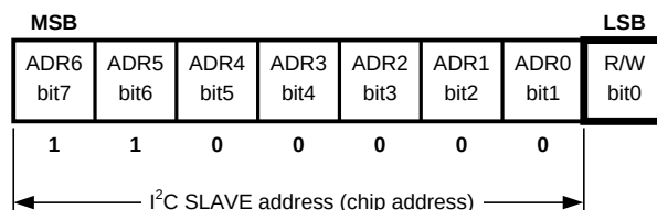
Figure 36. I 2 C Chip Address
