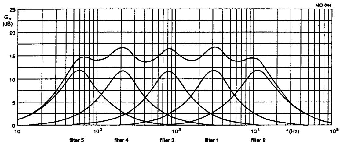
Fig.3 Frequency response for maximum boost of +12 dB according to Fig.1.
