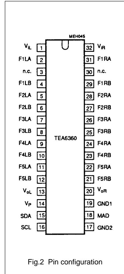
Fig.2 Pin configuration
