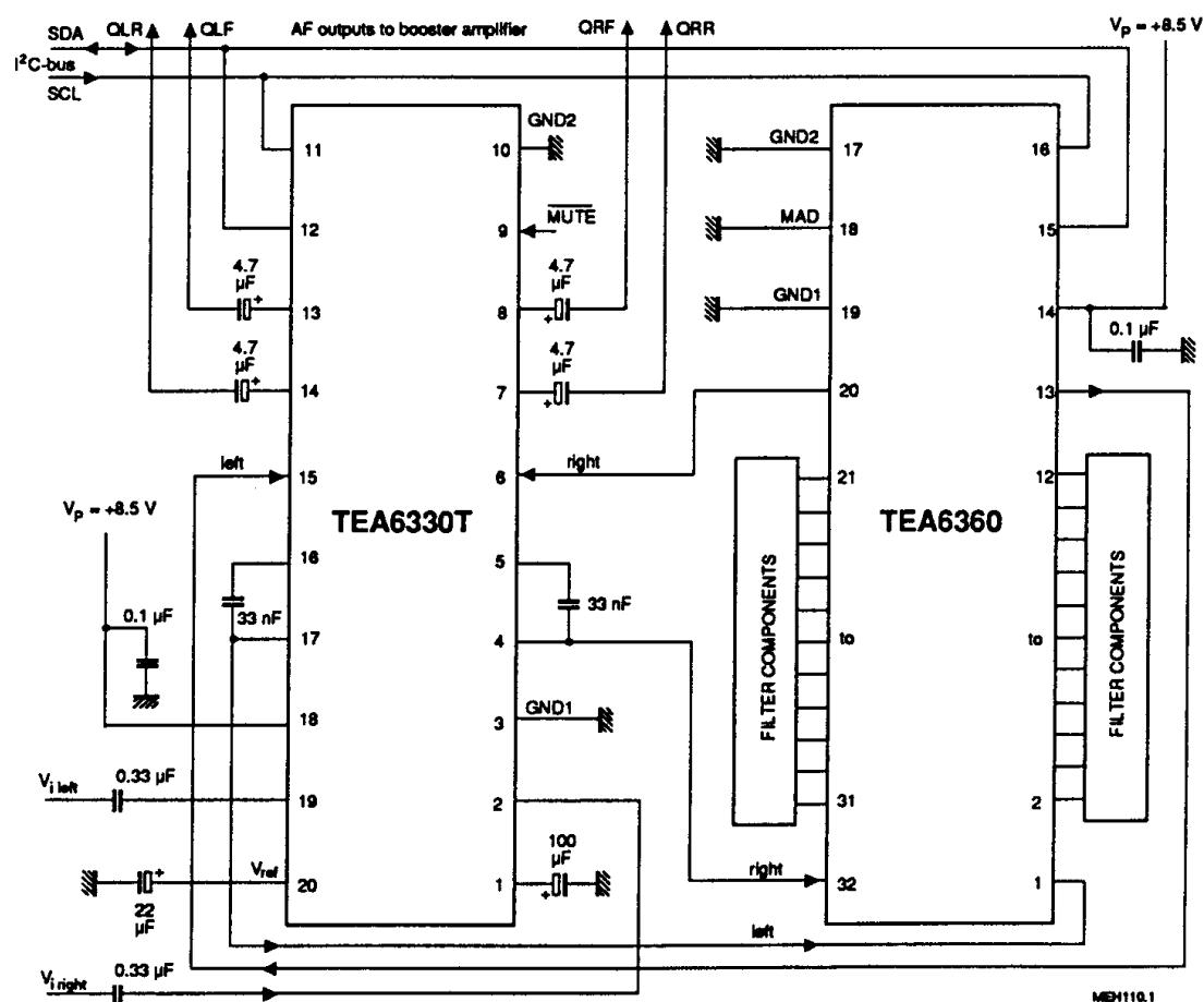
Fig.4 Application for car radio ( $V_p < 8.5$  V).
