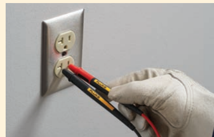
Increase tip exposure for CAT II probing
