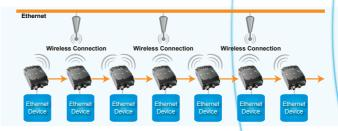
Wireless Ethernet Roaming. Here, WLAN /Bluetooth Ethernet Port Adapters connect to an Ethernet infrastructure via multiple Access Points. The WLAN Ethernet Port Adapters support several roaming modes including seamless roaming. We deliver superior wireless solutions. Nothing less.
