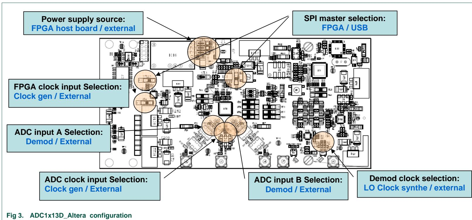
Fig 3. ADC1x13D\_Altura configuration
