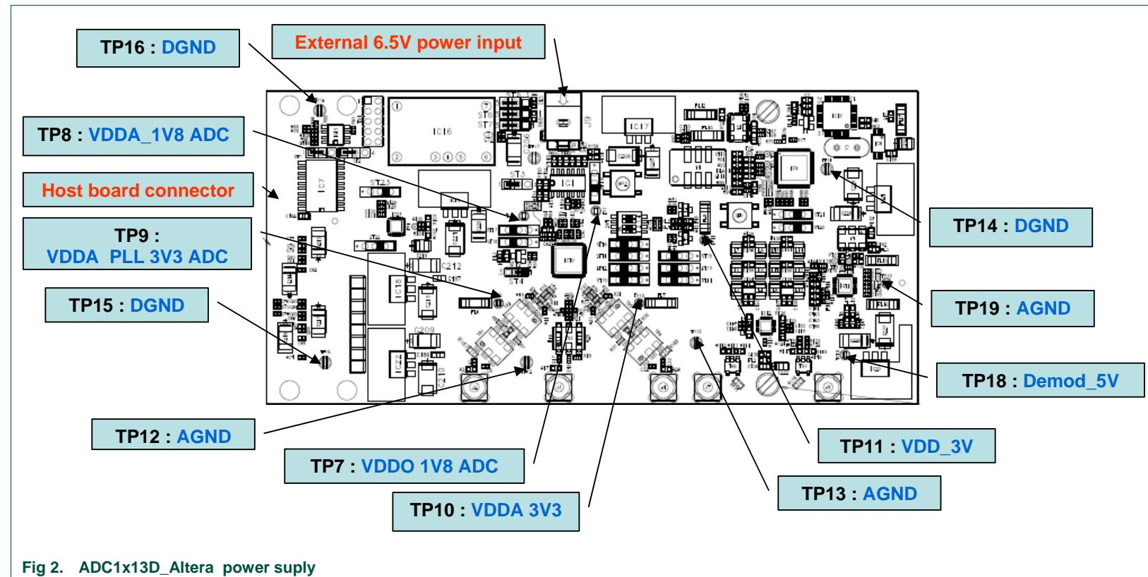
Fig 2. ADC1x13D\_Alttera power supply
