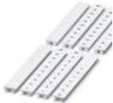
Zack marker strip, Strip, white, labeled, can be labeled with: Plotter, Printed vertically: Consecutive numbers 1 - 10, 11 - 20, etc. up to 91 - 100, Mounting type: Snap into tall marker groove, for terminal block width: 8.2 mm, Lettering field: 10.5 x 8.15 mm
