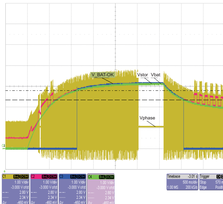
Figure 5. BAT_OK High/Low 2.8V/2.34V – Ramping Battery from 0V to 3.1V (0V) and Down to 1.8V.
