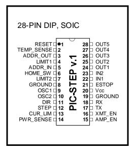
plus 5 undedicated outputs which can be used for amplifier control, or other purposes.
