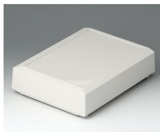
B4016657 Cover M, high ABS (UL 94 HB) off-white RAL 9002 6.61"x8.66"x1.97"
