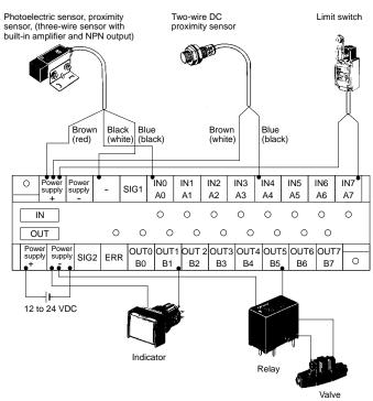
Note: IEC wire colors for photoelectric sensors and proximity sensors are shown first. The colors in parentheses refer to the old colors.
