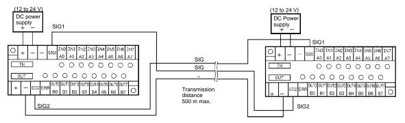
Note: A twisted pair or VCTF cable with a thickness of 0.75 mm<sup>2</sup> min. must be used for signal transmission.
