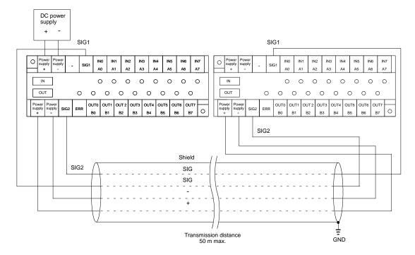
Note: In this example, a shielded transmission cable with a thickness of 0.75 mm<sup>2</sup> min. is used, through which a current of 1.8 A max. can be transmitted. It is recommended that the shield be grounded.
