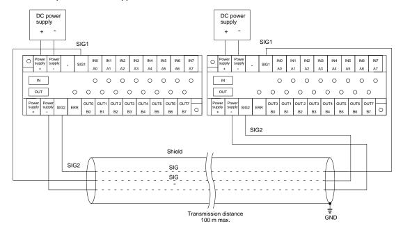
Note: A shielded cable with a thickness of 0.75 mm<sup>2</sup> min. must be used for signal transmission. It is recommended that the shield be grounded.
