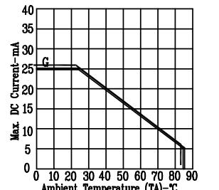
Fig5. MAX. ALLOWABLE DC CURRENT
