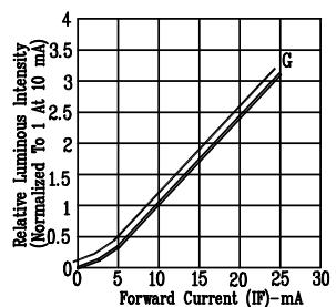
Fig4. RELATIVE LUMINOUS INTENSITY
