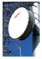
3.0 m | 10 ft Ultra High Performance Parabolic Shielded Antenna, dual-polarized, 5.925–7.125 GHz and 5.725 - 5.85 GHz, CPR137G, gray antenna, enhanced white radome with flash, standard pack—two-piece reflector
