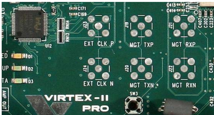
Figure 2-4: External Differential Clock Inputs
