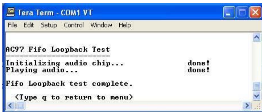
Figure D-17: FIFO Loopback Test Completion
