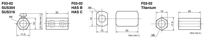
Note: 1. Dimension when mounting Electrodes.
