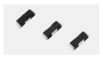
The VFM41R Series is an 1806 size, three terminal varistor-capacitor designed to remove ESD surges as well as provide EMI filtering. This filter provides excellent insertion loss characteristics exceeding 1GHz.
