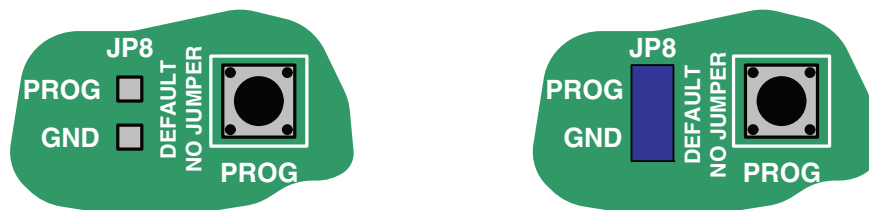
a) No Jumper: FPGA Operational (default)
