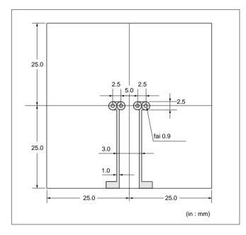
(2) Measurement condition Solder POSISTOR® on the substrate, then put the cover (150mm cubed) surround POSISTOR® to prevent flow of wind.
