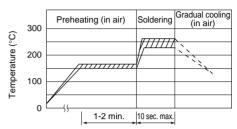
Preheating: 160±10°C, 1-2 min. Soldering: 230-260°C, 10 sec. max.
