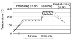
Preheating: 160±10°C, 1-2 min. Soldering: 230-270°C, 20 sec. max.
