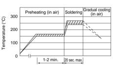
Preheating: 160±10°C, 1-2 min. Soldering: 240-270°C, 20 sec. max
