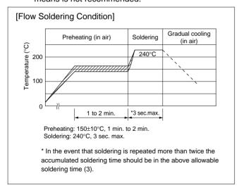
(5) There may be a risk of unexpected failures (tombstone, insufficient solder-wetting, etc.) in the mounting process caused by the mounting conditions. Please make sure that this product is correctly mounted under specified mounting conditions.
