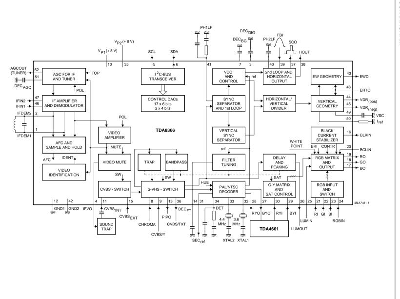
Fig.1 Block diagram (SDIP52; SOT247-1).
