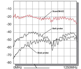
Frequency response of ScanEM-EC vs. passive probes.
