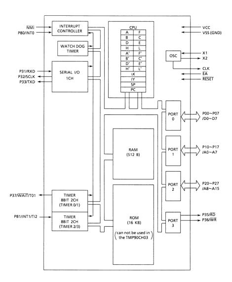
Figure 1. TMP90CH02 Block Diagram
