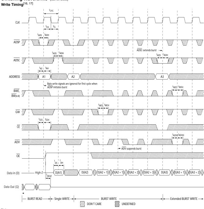
**Note:** 17. Full width write can be initiated by either  $\overline{\text{GW}}$  LOW; or by  $\overline{\text{GW}}$  HIGH,  $\overline{\text{BWE}}$  LOW and  $\overline{\text{BW}}_{[A:B]}$  LOW.
