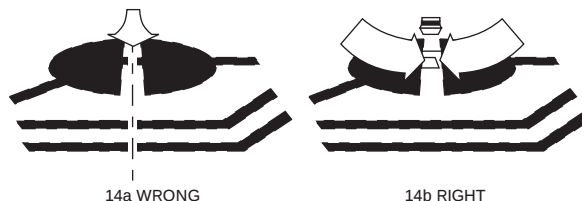
Figure 14 How to cut PCB links
