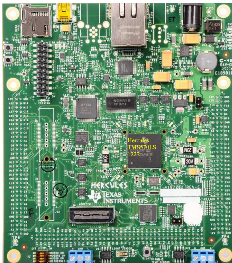
Figure 2-1. TMS570LS12 HDK Board, Interfaces Top Side
