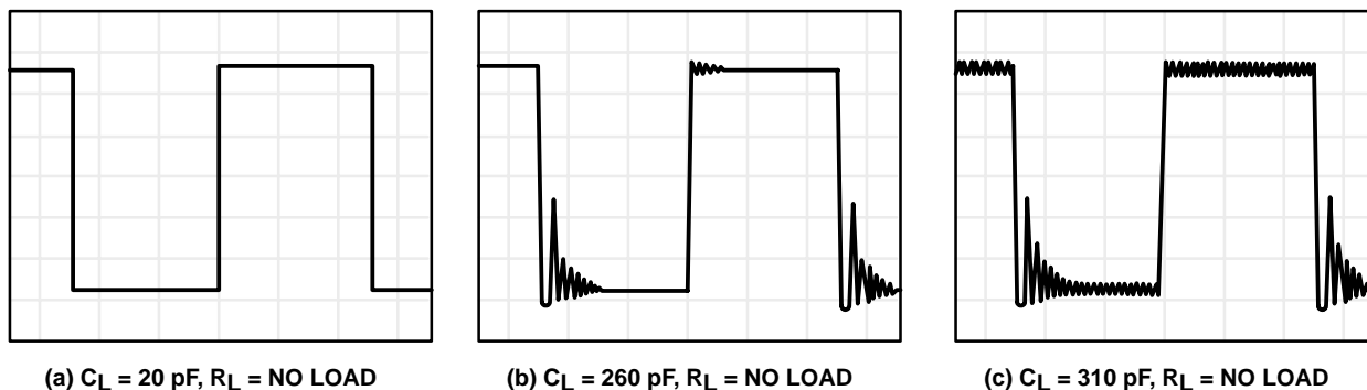
Figure 44. Effect of Capacitive Loads in Low-Bias Mode
