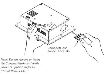
Information stored on a CompactFlash card by a G306A can be read by a card reader attached to a PC. This information is stored in IBM (Windows $^{\circledR}$ ) PC compatible FAT16 file format.
