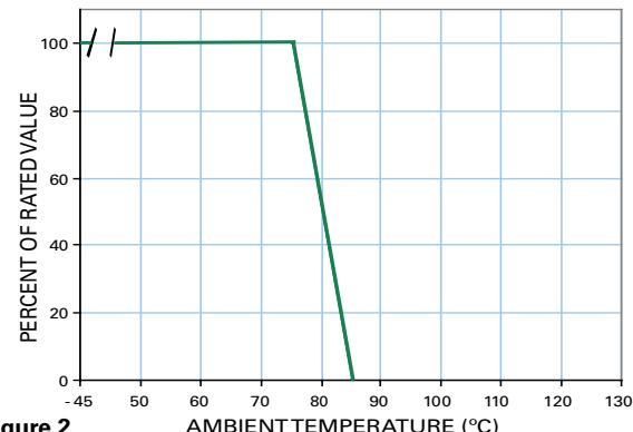
For applications exceeding 75°C ambient temperature, the peak surge current and energy ratings must be reduced as shown.
