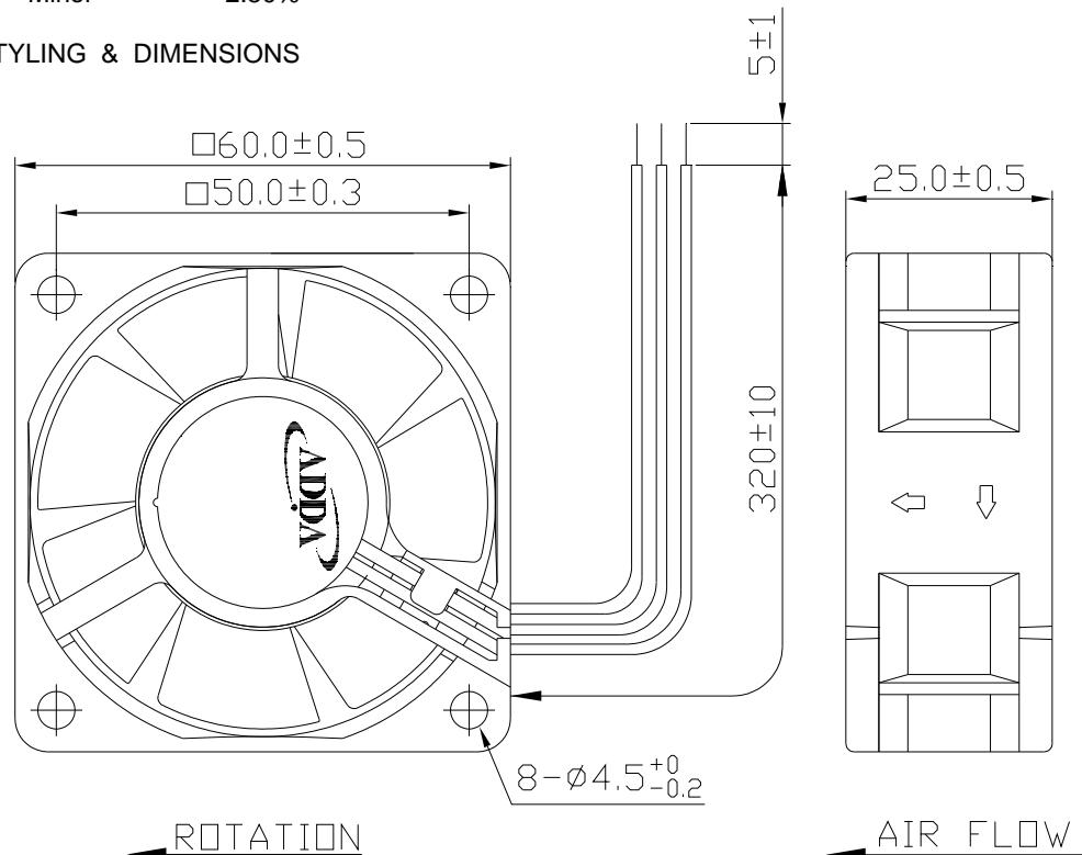
LEAD WIRES : UL 1007, AWG24, L = 320 +/- 10 mm
