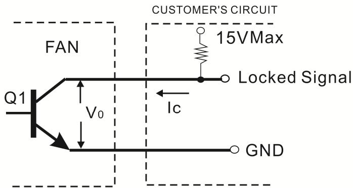
\*Transistor Q1 at "ON" position
