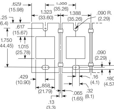
37D633 will mount eight solder terminal sockets in one length of aluminum strip measuring 10.97" x 2.25" x 0.062 (278.6 x 57.15 x 1.57)
