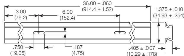
24A110 mounting track is designed to accept snap-mount sockets, as well as other P&B screw terminal sockets. Track is made of lightweight, sturdy extruded aluminum and is shipped in three-foot (914cm) lengths with mounting holes on six-inch (152mm) centers. Track can be cut to shorter lengths or used end-to-end.
