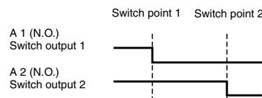
When  $A1 > A2$ , both switch outputs are activated as N.C. contacts.
