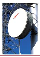
1.2 m | 4 ft High Performance Parabolic Shielded Antenna, single-polarized, 8.200–8.500 GHz, CPR112G, gray antenna, enhanced white radome with flash, standard pack—one-piece reflector
