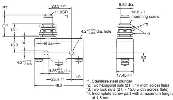
**Note:** 1. Do not use the M12 mounting screw and the case mounting hole at the same time, or excessive pulling force will be imposed on the switch and the case and cover may be damaged.
